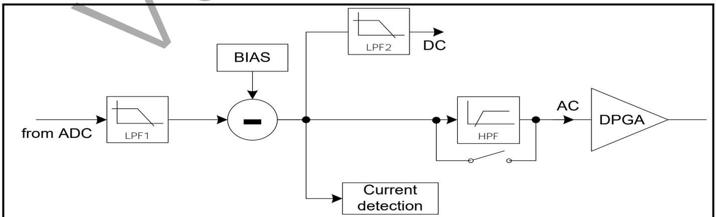
Figure 8-2 Signal Processing for Current Detection
