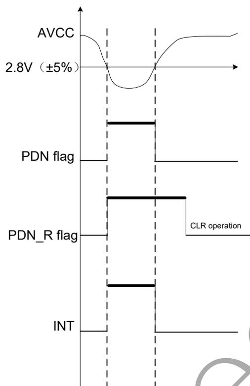
Figure 4-2 Power-Down Interrupt
