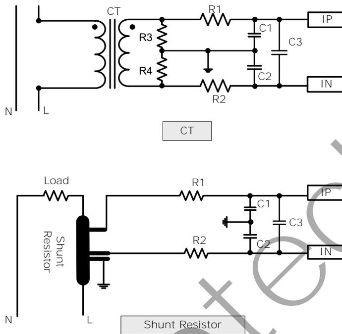
Figure 7-2 Analog Input of Current Channels
