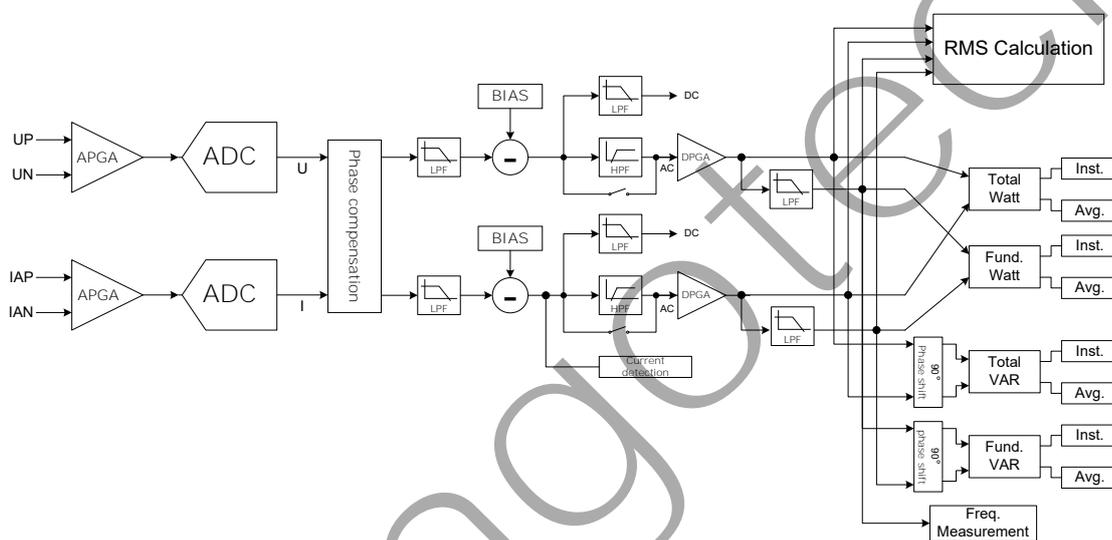
Figure 7-1 Signal Processing in Specific Metering Architecture
