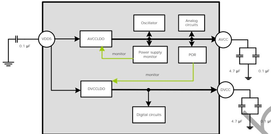
**Figure 4-1 Power Supply Architecture**
