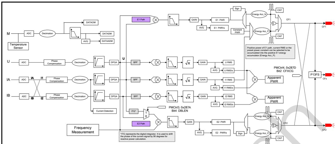
Figure 10-1 Digital Signal Processing in Vango Metering Architecture
