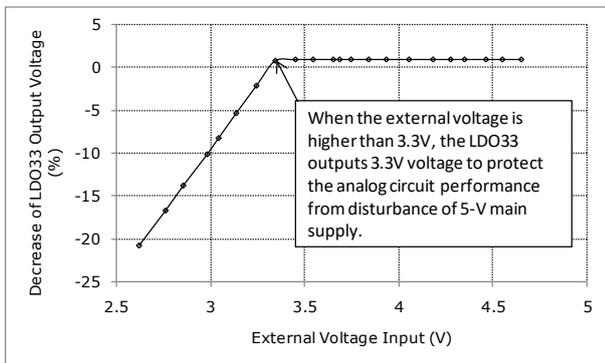
**Figure 8-2 LDO33 Output and 5V Power Input**
