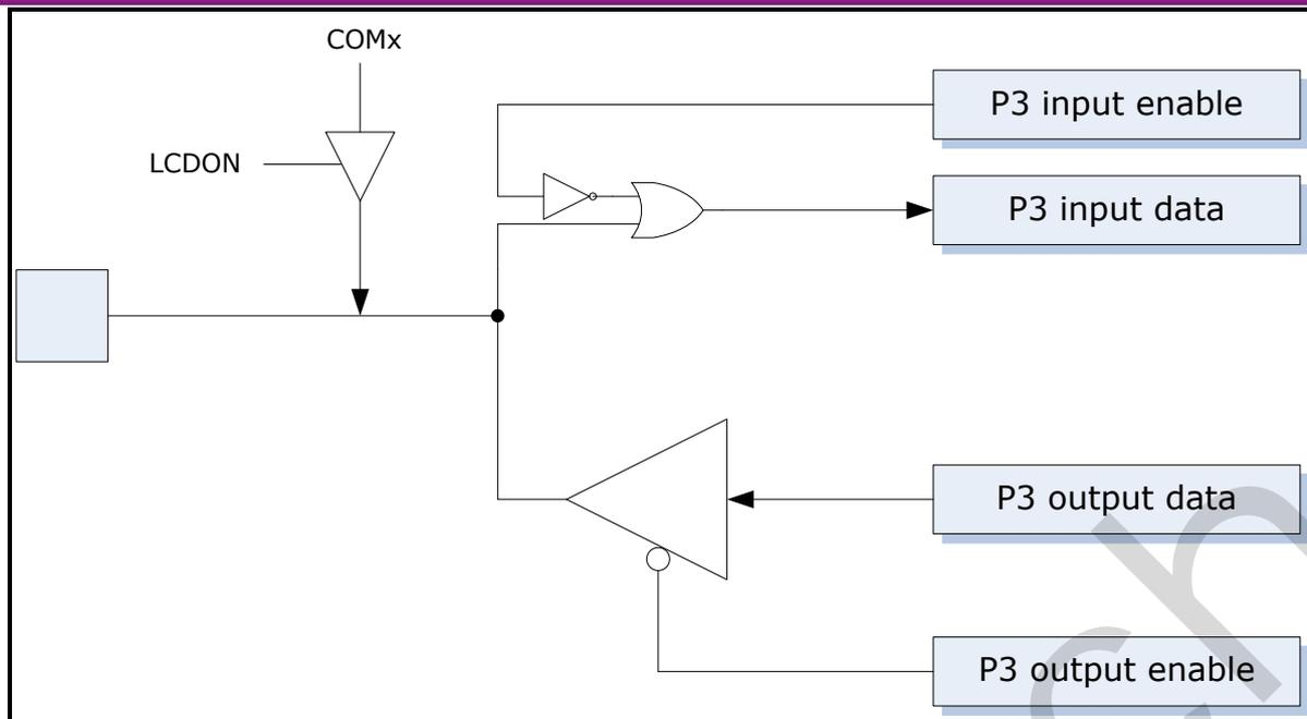
Figure 15-5 Architecture of Each Port of Group P3
