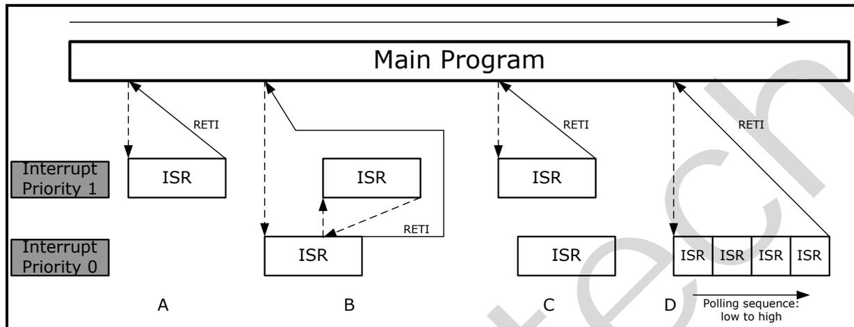
Figure 11-2 Interrupt Processing
