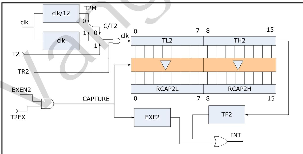
Figure 12-10 Timer2, 16-bit Timer/ Counter in Capture Mode
