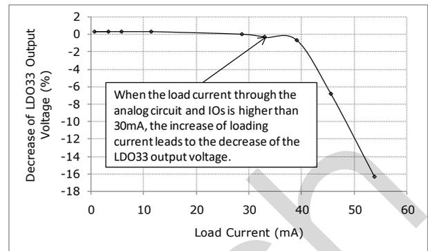
**Figure 8-3 LDO33 output and the Load Current**
