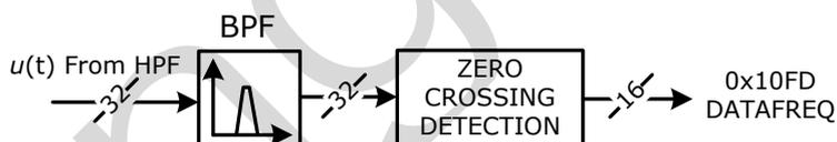
Figure 10-13 Signal Processing for Line Frequency Measurement
