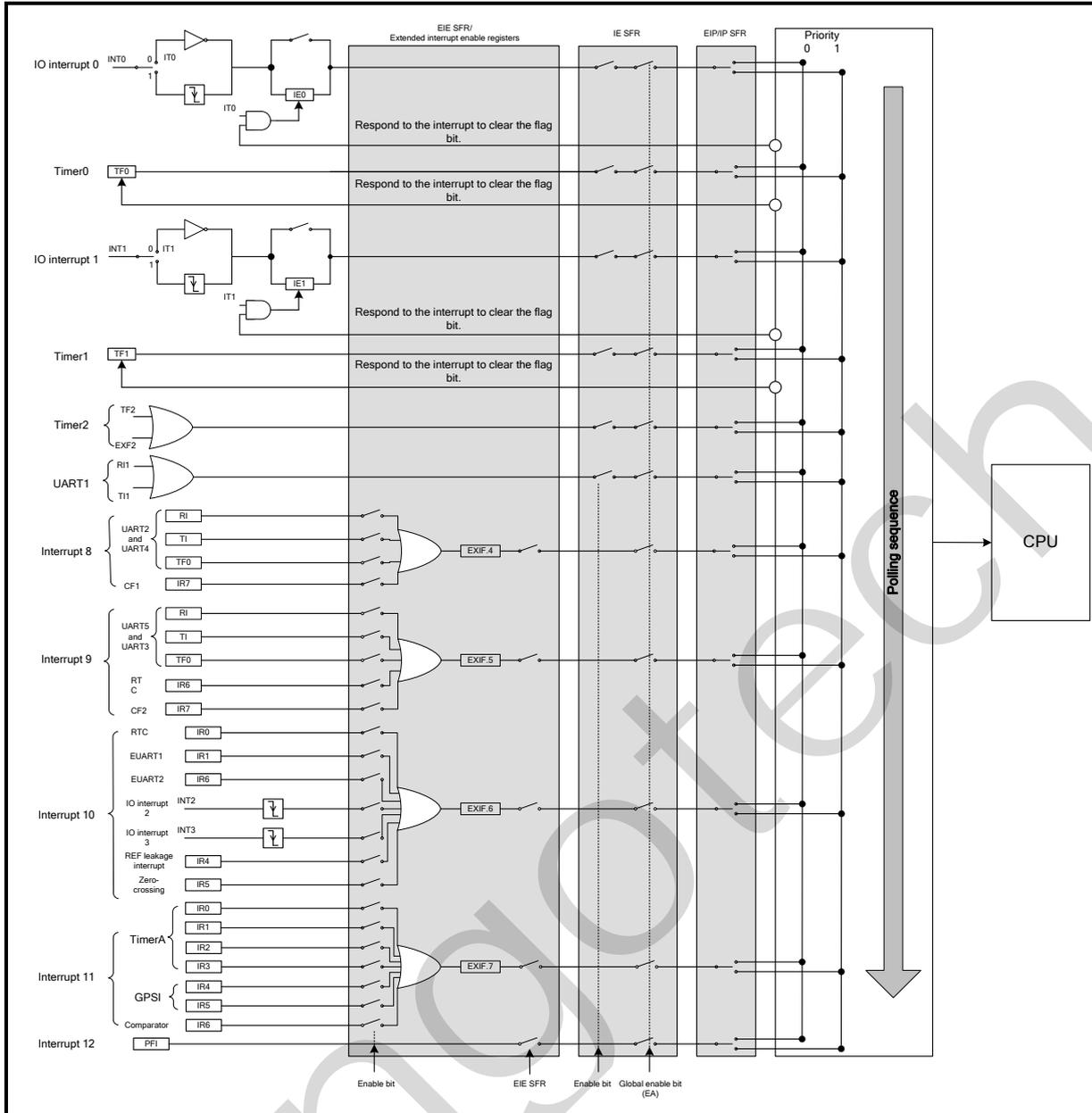
Figure 11-1 Interrupt Logic
