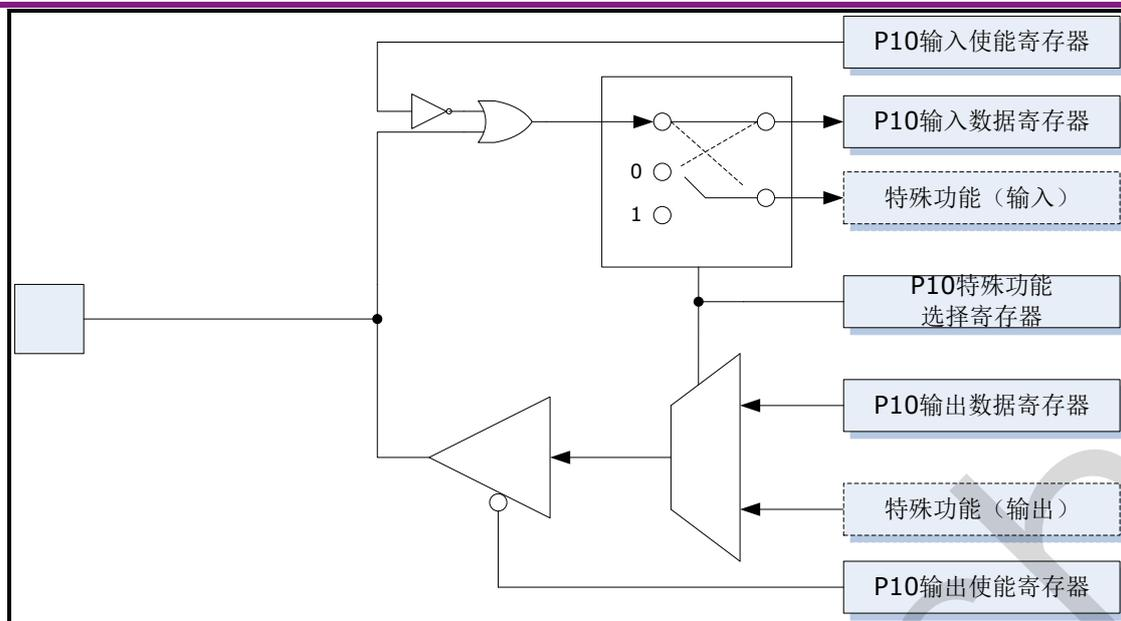
Figure 15-12 Architecture of Each Port of Group P10
