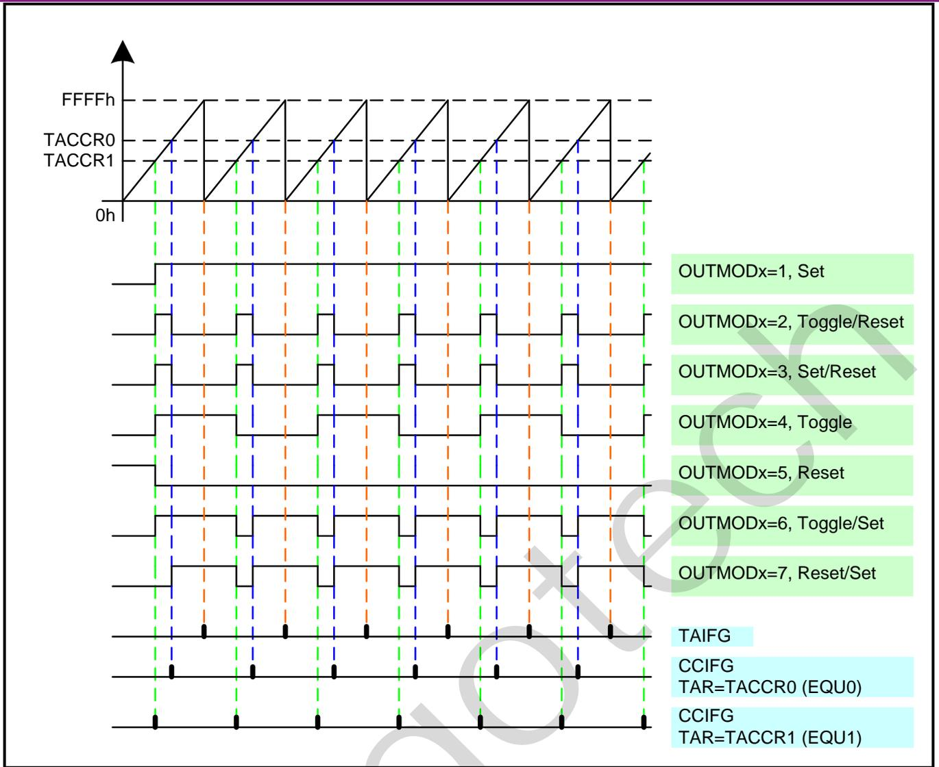
Figure 12-5 Output on Pin TA1 in Continuous Mode
