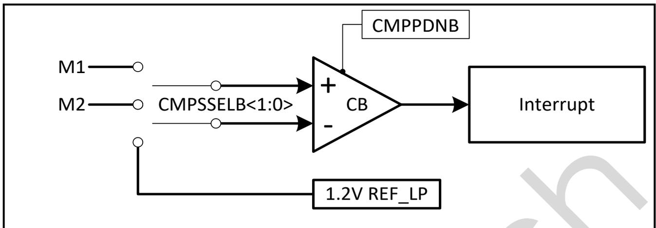
Figure 9-1 Comparator Architecture
