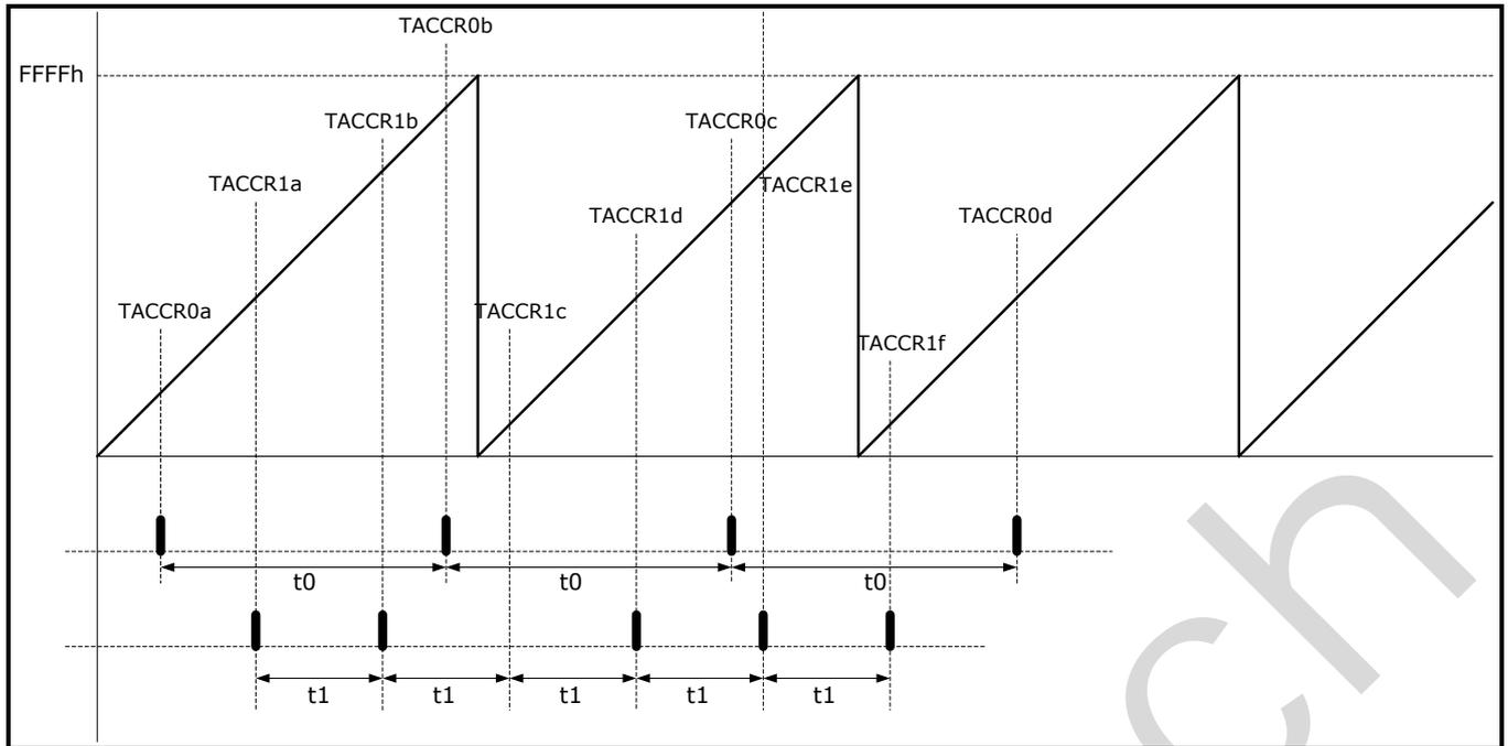
**Figure 12-3 Configuring Output Frequency in Continuous Mode**
