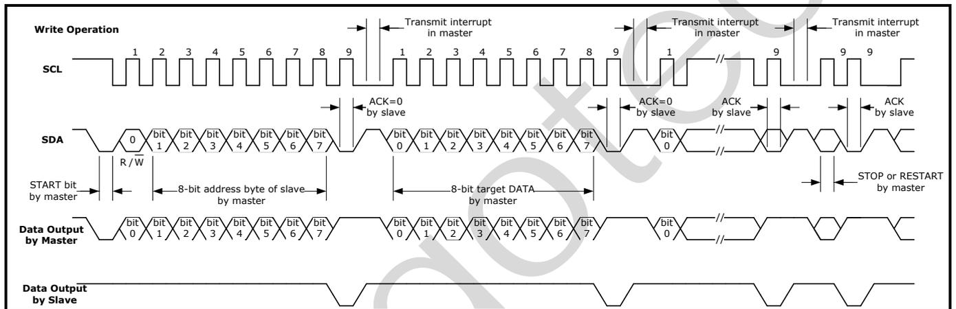
**Figure 13-4 Write Operation**
