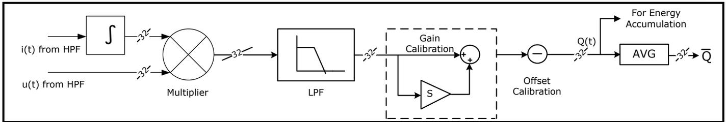
**Figure 10-11 Signal Processing for Reactive Power Calculation and Calibration**
