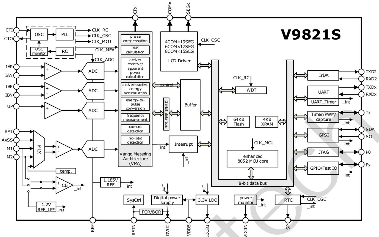
\*1.2V REF\_LP represents the low power reference voltage unit (not the BandGap circuit). This unit works all the time until the chip is powered off. This unit provides the 3.3V LDO and digital power supply with 1.2V reference voltage, and it can be the negative input for the comparator CB.
