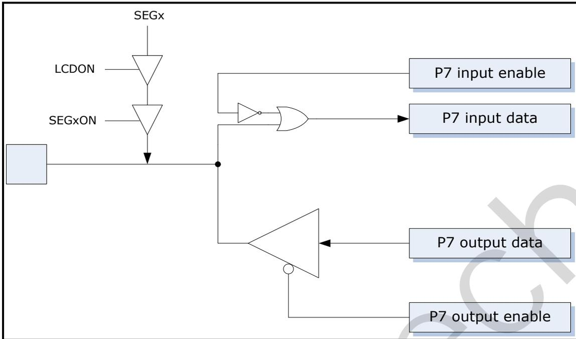
Figure 15-9 Architecture of Each Port of Group P7
