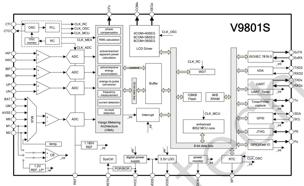
\*1.2V REF\_LP represents the low power reference voltage unit (not the BandGap circuit). This unit works all the time until the chip is powered off. This unit provides the 3.3V LDO and digital power supply with 1.2V reference voltage, and it can be the negative input for the comparator CB.
